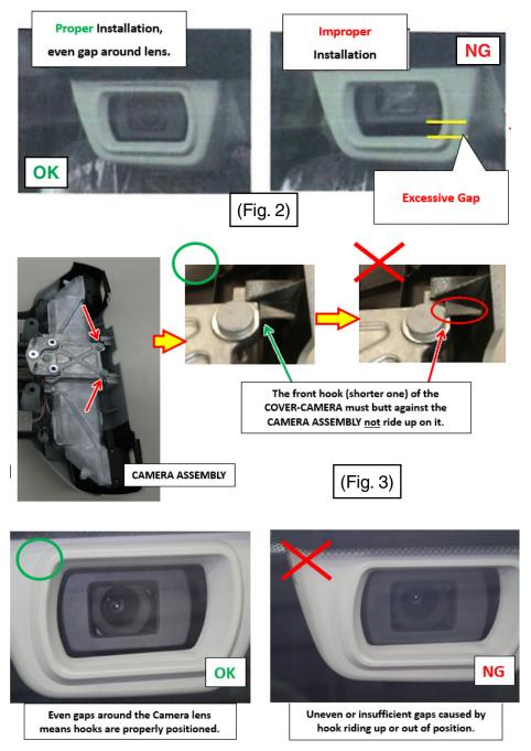
**VERY IMPORTANT:** Whenever the camera cover has been removed, always confirm proper EyeSight system operation as a final quality check before releasing the vehicle.
