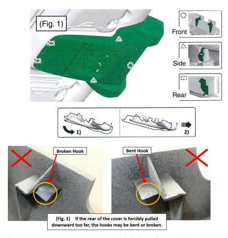
When reinstalling the camera cover, **CAREFULLY** slide it from front to back to engage the two front hooks first followed by the side clips then the rear clips.
