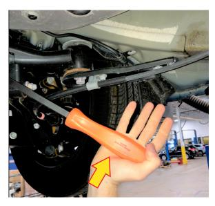
If the weld is broken, cracked or at all damaged and the base metal is exposed, replace the rear subframe with a new part. If the weld is OK, always make sure to touch-up any paint damage from the pry bar. Wipe the area clean with mild solvent on a fresh shop cloth, allow to dry then apply rustpreventative touch-up\*\* to prevent corrosion.
