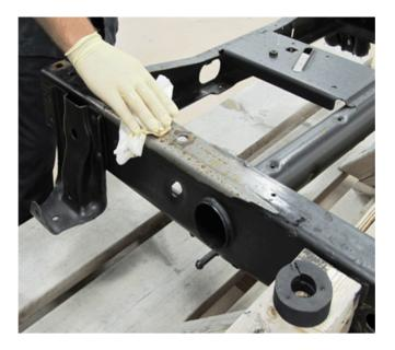
8. Using Lloyd's Pure Prep™ Metal Surface Preparation P/N 25418 (10 fluid ounce bottle), or equivalent, saturate a towel or Scotch-Brite™ (3M) pad with the pre-diluted solution and scrub the area well, rendering a foaming of the Pure Prep.™ This will greatly improve adhesion and corrosion resistance in the repair areas.
