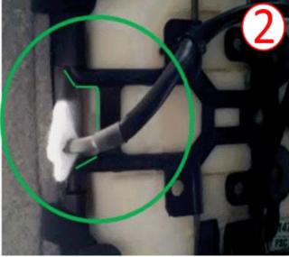
**Note:** The graphic above depicts the incorrect pigtail harness route (1) and the correct pigtail harness route after repair (2).
