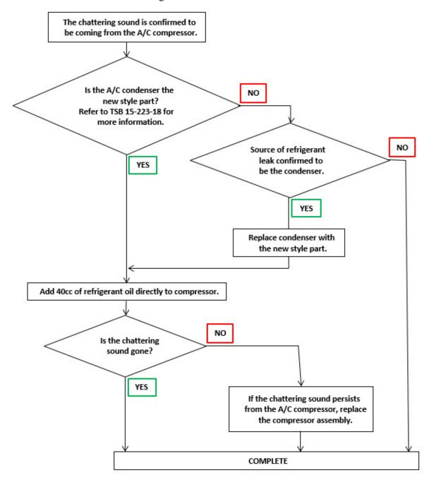
When adding oil directly to the compressor there are two (2) methods:
