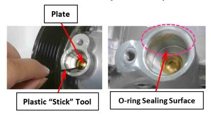
• **CAREFULLY** add the measured amount (40cc) of refrigerant oil. Turn the armature of the compressor CLOCKWISE while filling as needed.
