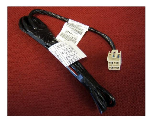
2. Connect the harness to the MID-BEC (X61A). The MID-BEC is located under the I/P to the left of the steering column. The harness connection point (1) is illustrated below.
