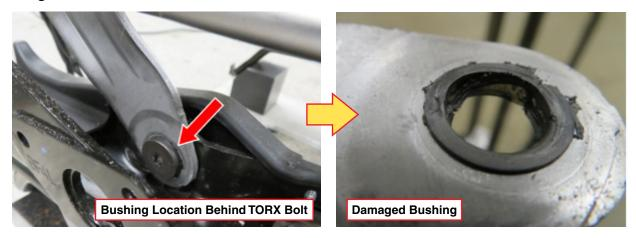
**NOTE:** Only inspect one side at a time. If OK, re-install the TORX bolt and retorque to  $15 \pm 2$  Nm (11 ft. lbs.). Most damaged Teflon bushings are found on the inboard side.
