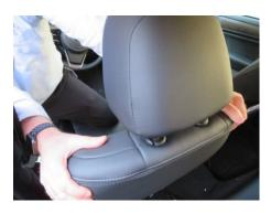
**Step 2-** While sitting in the rear seat, apply back and forth pressure to the backrest while pushing downward toward the seat frame slide rails. Repeat this step using a twisting motion. This applies pressure to the TORX bolts and will help isolate any squeaks.
