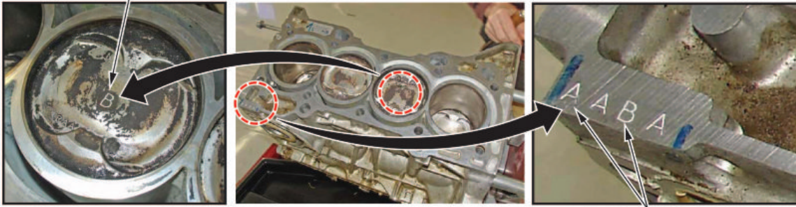
The "A" and "B" represents piston size. Piston sizes can be mixed in an engine block assembly.
