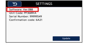
If a different SETTINGS screen appears, touch the "General" tab. Otherwise press the Version soft key on the screen to display the unit's current software version.
