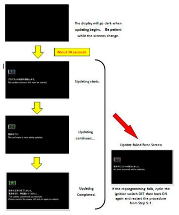
• **IMPORTANT:** Do not remove the USB flash drive or turn the ignition off while software is updating. The updating procedure will take approximately 10-12 minutes to complete.
