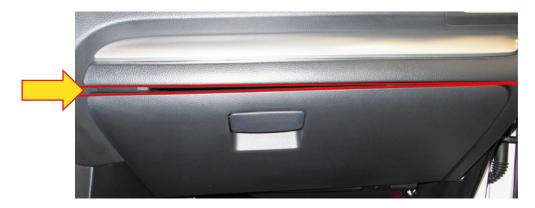
There is a latch to keep the glove box closed on both sides of the glove box door. If the door is closed without using enough force to engage both latches or by pushing it shut on just one side instead of in the middle, one may close and not the other. Over time, if the door is not fully closed with both latches, high cabin temperatures along with weight of the items inside the glove box may cause the assembly to deform slightly and a gap to develop.
