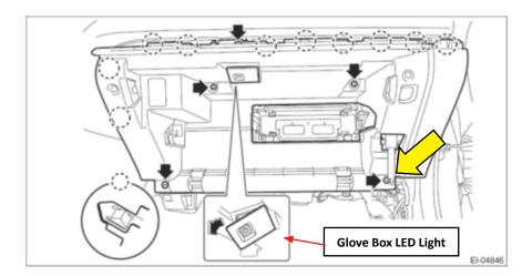
• Start by installing one flat washer as a shim between the back side of the inner panel and the support beam. Place an inner panel retaining screw back into the hole indicated by the yellow arrow then put the washer on the threaded portion. As an alternative, use a small piece of tape to hold the washer in place on the support beam while refitting the inner panel. The yellow arrow on the illustration below indicates the screw hole where the shim belongs.
