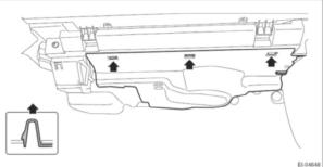
• Using a plastic trim tool, release the clips and remove the instrument panel trim and end cover.
