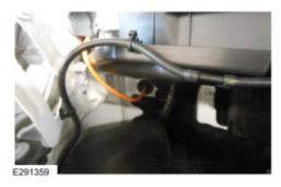
**21.** Route the orange antenna wire in front of the deflector and route the washer hose under the inboard end of the deflector. Attach the washer hose clip to the front edge of the deflector. (Figure 7)
