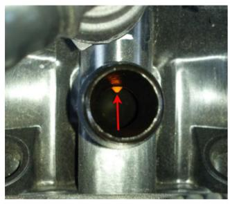
If the non return valve is not visible as shown in picture, then use a long cotton swab to wipe any excess oil from the valve to validate.
