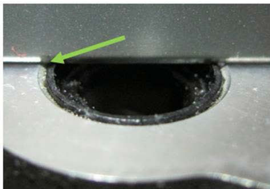
OK- Filter Screen flush with machined surface of camshaft carrier.
