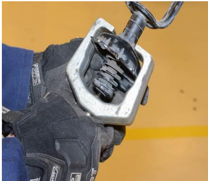
Fig. 2 Puller Correctly Installed On Seat
