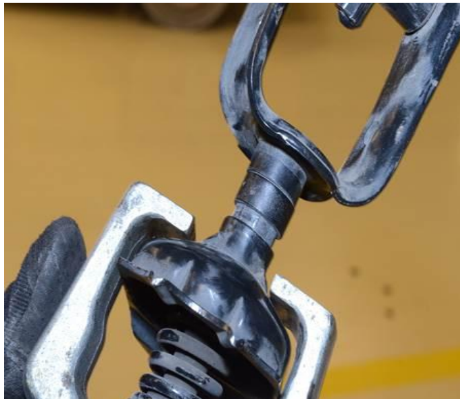
Fig. 3 Spring Compressed On Seat
