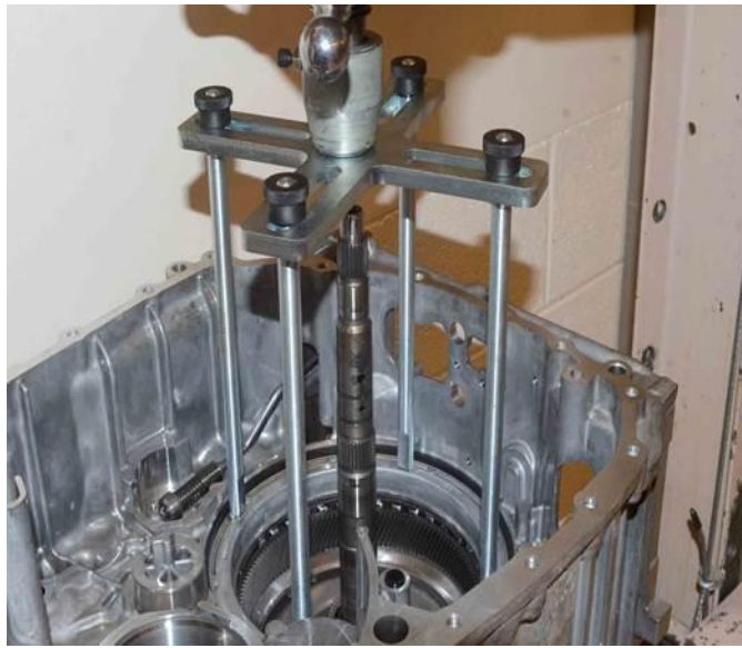
Fig. 8 Pressing Tool Installed
