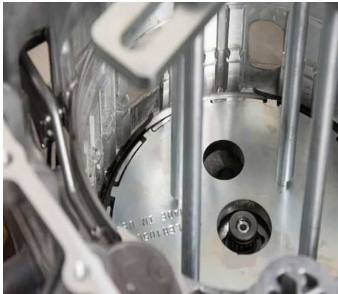
Fig. 11 New Snap Ring Installed
