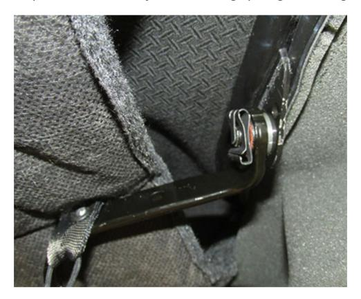
The folding top linkage that attaches to the rear glass MUST be located on the outboard side of the back glass bracket.
