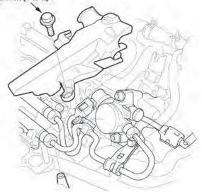
27. Install the intake base and intake manifold.
