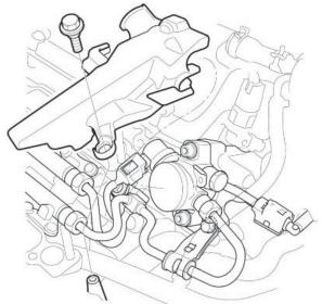
5. Remove the quick-connect fitting cover.
