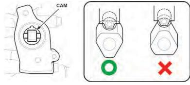
17. Coat the roller, O-ring, cam and around the bore of the lifter with clean engine oil.
