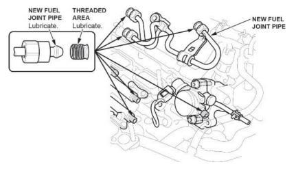
20. Tighten the fuel joint pipe nuts by hand until the end of the joint pipe is seated on the fuel rails and high pressure fuel pump.
