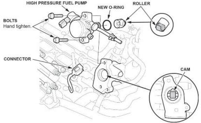
18. Install the roller and the high pressure fuel pump. Install the bolts loosely by hand in an alternate pattern. Connect the connector.
