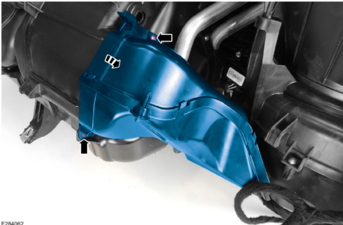
8. Remove the 2 heater core outlet pipe cover fasteners from the climate control housing and remove the cover. (Figure 7)
