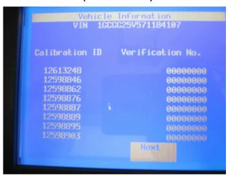
If the Tech 2® that is being used displays all zeroes for the Verification Numbers as shown, then perform the following steps:
