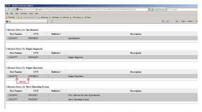
Compare each: Engine Calibration Part Number History parameter and Calibration Verification Number History parameter from the GDS 2 Calibration History screen to the Calibration Part Number and Calibration Verification Number (CVN) listed in the GM Vehicle Calibration Information screen of TIS2WEB to ensure that they are ALL an EXACT MATCH.
