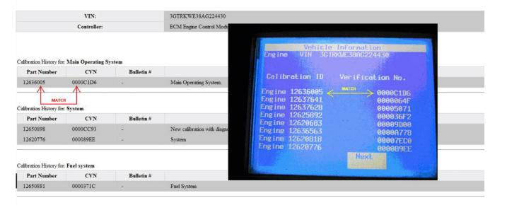
Compare each: Calibration ID Part Number and Verification No. (Number/CVN) from your Tech 2® photo to the corresponding Calibration ID Part Number and Verification No. (Number/CVN) listed in the TIS2WEB GM Vehicle Calibration Information screen of TIS2WEB to ensure that they are ALL an EXACT MATCH.
