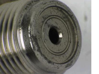
If additional debris that can NOT be picked up with a magnet (Contamination) is found on the Fuel Pressure Regulator 1, Fuel Rail Pressure Sensor, and/or Fuel Pressure Regulator 2 (Pressure Relief Valve), refer to PIP5370 and Contaminants-in-Fuel Diagnosis. DO NOT perform the repair listed in this bulletin.
