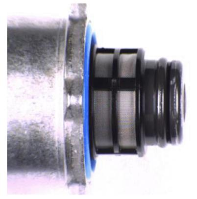
If Pressure Regulator 1 has no debris that can be picked up with a magnet on the screen, continue with Fuel Injection Pump replacement.
