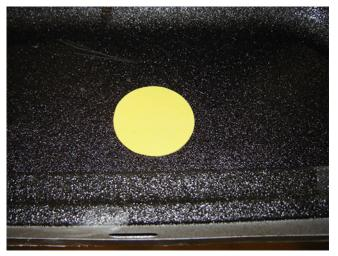
7. Place the textured pad over the repair area and apply firm and even pressure for a minimum of 2 minutes.
