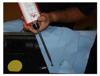
5. Purge the mixing tip away from the repair area (on the towel) to ensure proper material mix. Pump the cartridge at least 3 times verifying there are no striations in the material to ensure proper mix. The material should be a solid black color.
