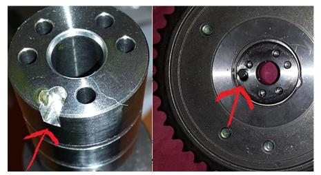
Replace and or repair the rockers, SHLAs, DF SHLAS, actuator and camshaft as needed per damage found.
