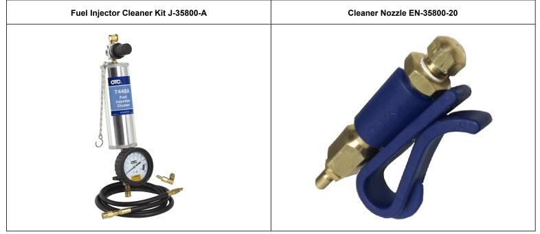
Important: Extreme care must be taken not to hydro-lock the engine when inducing the cleaner, especially if it is induced without Fuel Injector Cleaner Kit J-35800-A or equivalent. If too much cleaner is induced at too low of a RPM, or if you force the engine to stall by inducing too much cleaner at once, the engine may hydro-lock and bend a connecting rod(s).
