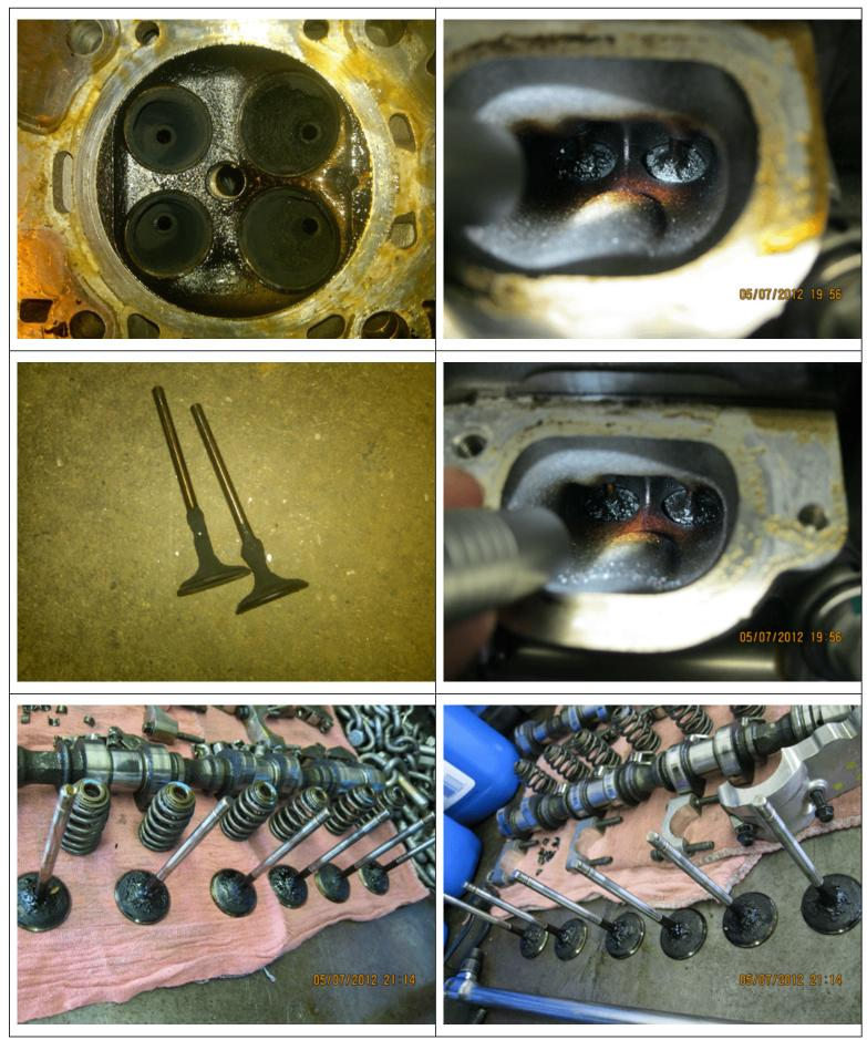
When the engine is cold, the compression on multiple cylinders may be at 0 PSI (0 kpa). The engine also may pop through the intake or exhaust while cranking and the spark plugs may be fuel fouled when inspected. Some engines may also experience valve damage or cam followers that are out of position as a result of this.
