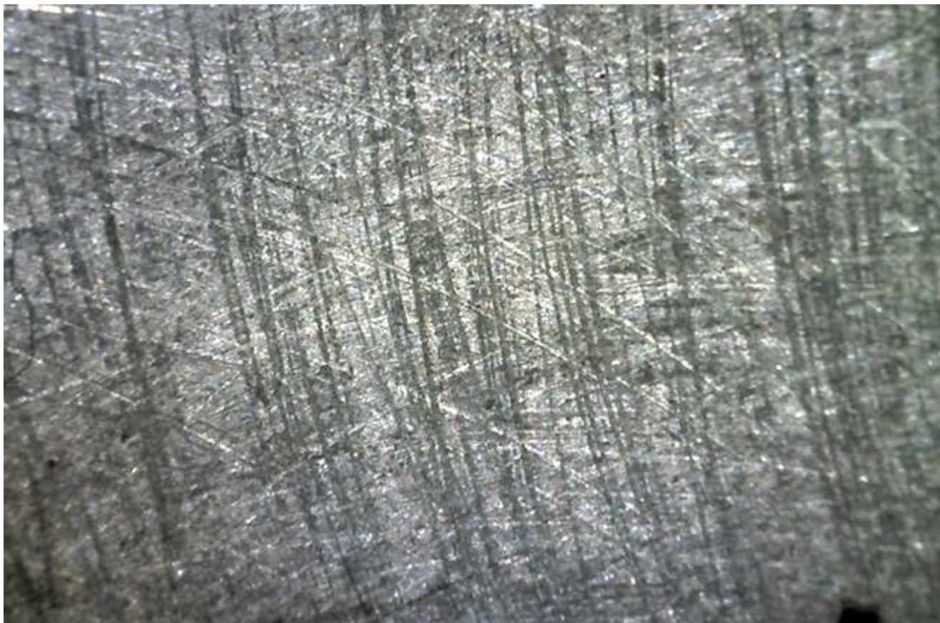
A close-up of the surface shows deep grooves caused by use of a wire wheel.
