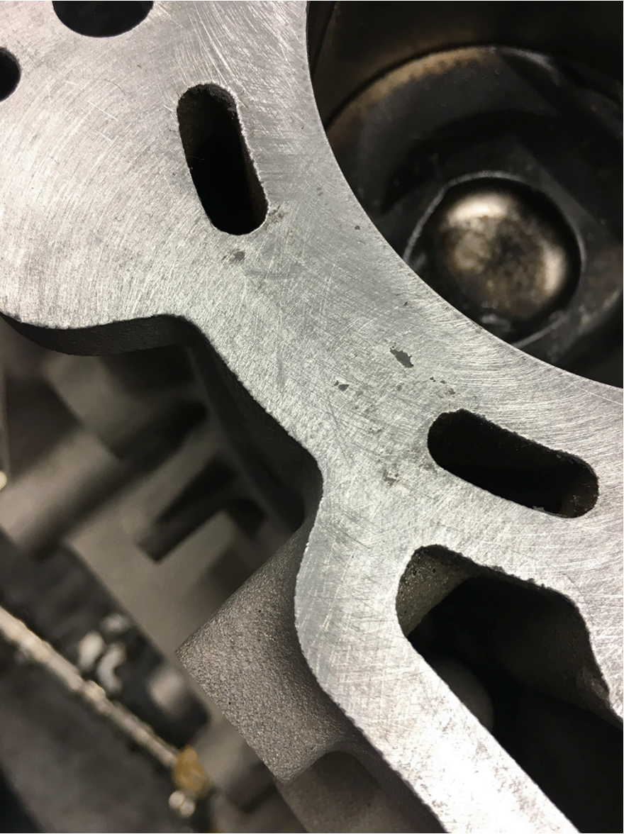
An overview of the deck face when it has been cleaned with an abrasive pad, left swirls on the surface and do not go in the same direction which caused changes the surface dimensions (flatness) of the block leaving it un-usable.
