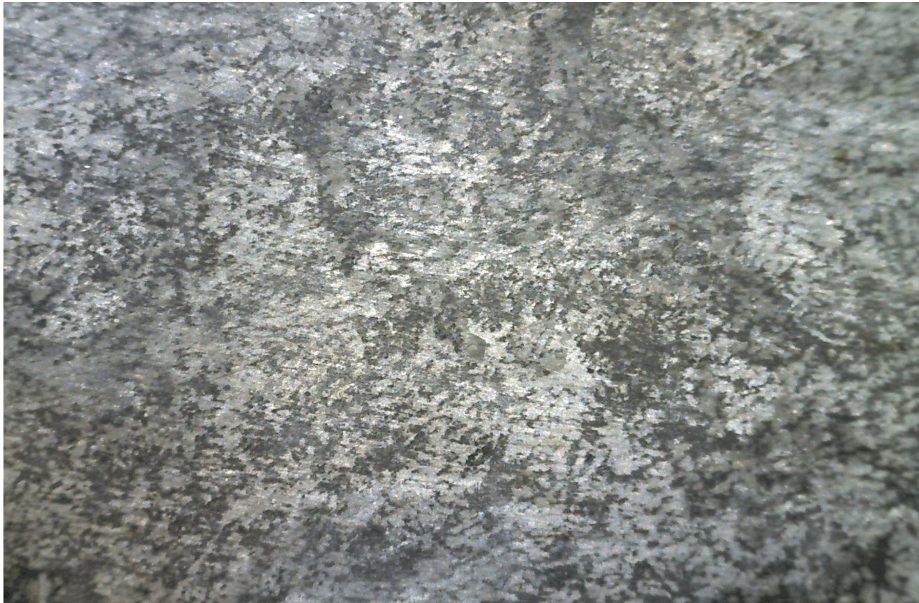
A close up of the sealing surface after cleaned with GM Low VOC Cleaner and plastic scraper.
