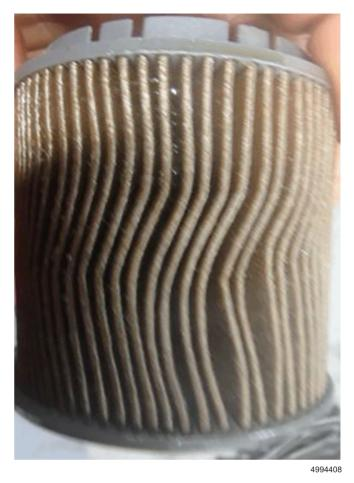
Shown are oil filter pleats with visible metal particles. In this example, minimal amounts of metal particles are visible on oil filter pleats and should not pose a concern.
