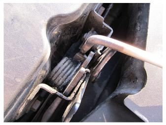
3. Rotate the release tool counterclockwise to push release lever.
