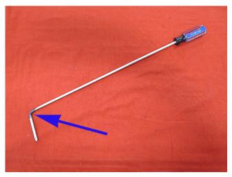
3. Clamp the screwdriver in a vise and create a 90° bend as shown.
