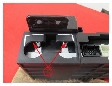
Remove the illustrated sections (1) of the bracket to allow the module's connectors access.
