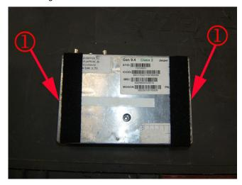
Install one side of 2" Velcro® 191195 Reclosable Loop Fastener Tape (hook and loop) or equivalent as shown above to the new OnStar® module.
