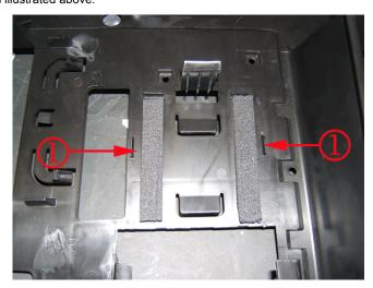
Install the OnStar® module and secure the module with nylon wire tie as illustrated. Trim the excess wire tie material.
