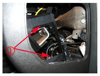
Install the other side of the 2" Velcro® 191195 Reclosable Loop Fastener Tape (hook and loop) or equivalent to the OnStar® module bracket as illustrated.
