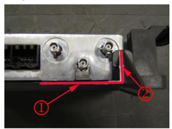
Remove only enough material from the lower edge (1) and shoulder (2) from the bracket to allow the module to seat fully. Continue with the installation procedure.
