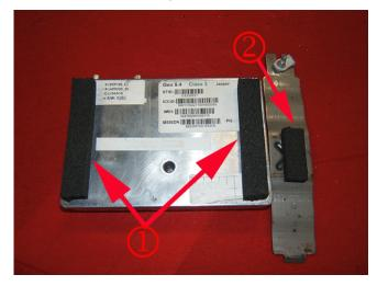
Install two strips of Kent Automotive Adhesive-Back Shim Stock 3/4" Wide X 7/16" thick or equivalent to the bottom of the OnStar® module and install a piece of foam (2) to the locking strap as illustrated.
