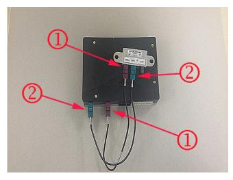
**Note:** During installation of the antenna cable and the cellular cable to the splitter, if the cables inadvertently become incorrectly installed, the techniciar may notice a red LED with DTCs B101D-3C and B101D-F0 set as current in the OnStar VCIM.
