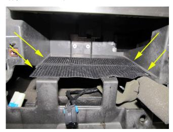
3. In the open space in the instrument panel (I/P), where the original module was, install on the bottom portion of I/P the other side of the 2" Velcro® 191195 Reclosable Loop Fastener Tape (hook and loop) or equivalent as shown above.
