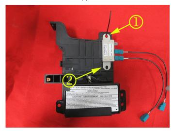
Secure the splitter to the side of the bracket as illustrated above.
