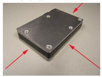
Wrap the new module with Scotch™ Linerless Rubber Splicing Tape 130C, 19 mm (¾ in) wide, (rubber tape) or equivalent from left to right, covering the back side of the module as illustrated.
