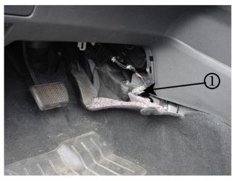
2. Locate the HO2S connector (1). Clean the connector with compressed air and apply a small amount of silicone grease to the connector.
