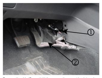
Remove the side IP panel (1) then move the carpet back to gain access to the HO2S connector.
