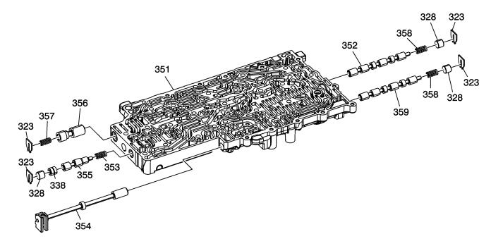
During inspection of the Clutch Select Solenoid Valve 2 (359), the valve may or may not be stuck in the bore due to the valve body bolts being loosened.
