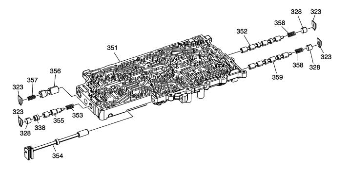
This condition may be caused by the Clutch Select Solenoid Valve 2 (359), located in the lower valve body, sticking in its bore resulting in a 4th gear start.
