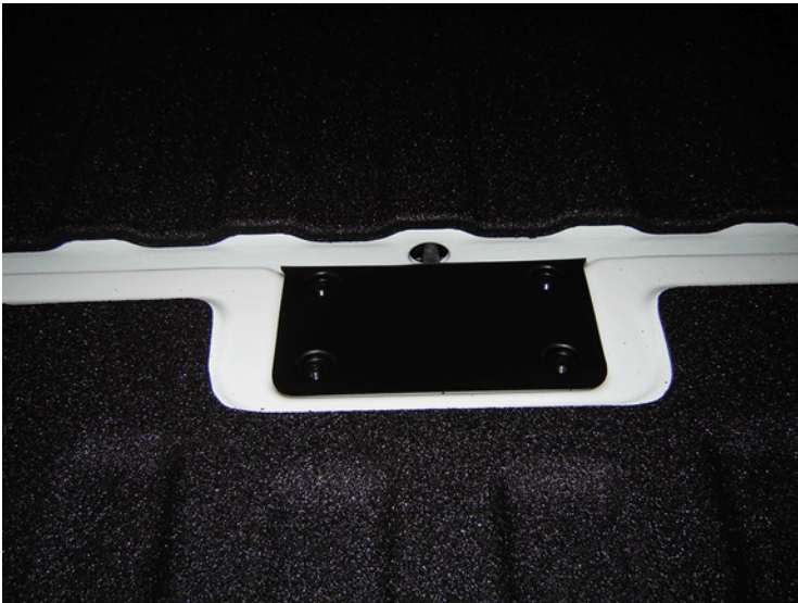
Bed floor (with rear camera access panel, gate open)
