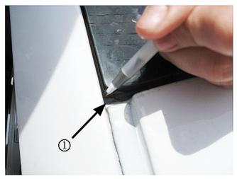
4. Also inspect the forward-most edge of the ditch, assuring any gaps in the factory sealer are filled. Inspect and seal all the way to and below the rubber windshield lace (1).
