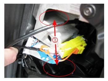
• Remove the IP outer trim cover and inspect for water/spotting within the end opening on the IP (1).
