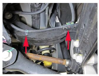
3. Release the two harness retainers from the control arm.
