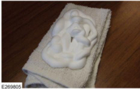
6. Apply a layer of Motorcraft® ZC-54 Professional Strength Carpet and Upholstery Cleaner or equivalent to the water stained area(s) of the headliner and allow to soak for one minute. (Figure 4)
