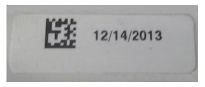
If the date on the sticker adhered to the backside of the Outside Rearview Mirror Charge Status Indicator LED Lens assembly is earlier than June of 2014, the Outside Rearview Mirror Charge Indicator LED Lens assembly will need to be replaced.
