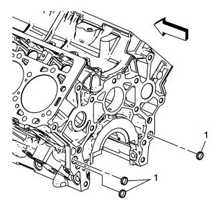
If one oil gallery cup plug is found to be leaking, replace all three (two on the left and one on the right) cup plugs at the same time the flywheel housing is resealed.
