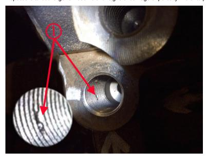
2. Inspect for imperfections in the gasket sealing surfaces (lack of flatness, debris or damage to the feed line banjo fitting itself.)
