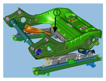
Note: The height adjuster motor is always on outboard side of cushion adjuster.
