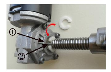
To eliminate the manufacturing variation, add a split washer/retainer to the drive screw between the interface of the motor casting (1) to the spindle nut (2). The graphic above shows the height adjuster motor with the retainer added, and another sample retainer alongside the motor.
