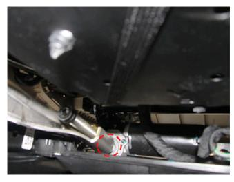
**Note:** Depending on vehicle model, the retainer can be installed from the front or the rear, however in most cases it may be easier to visually see the install location from the rear.
