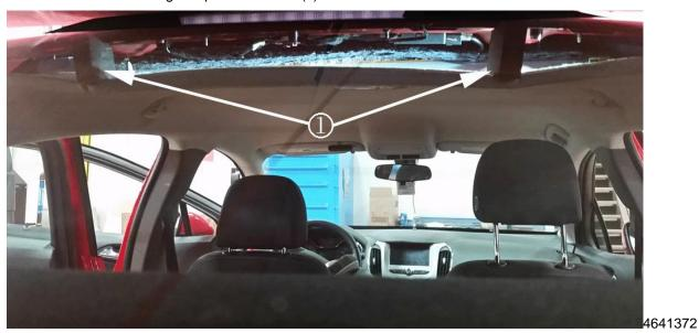
20. Install two foam blocks (1) between the roof of the vehicle and the headlining trim panel to gain access to the high mount stop lamp nuts.
