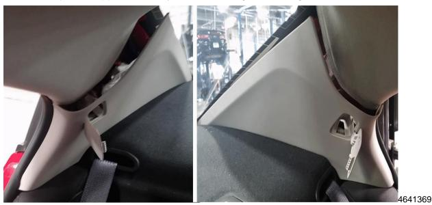
**Note:** It is NOT necessary to remove the lower fastener from the body side rear window garnish moldings.
