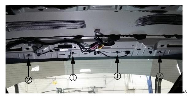
Note: The two middle high mount stop lamp nuts (1) MUST be torqued first.
