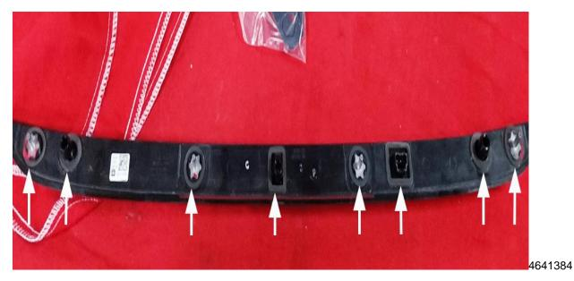
**Caution:** Do NOT use sharp tools or any chemicals to remove the gaskets from the high mount stop lamp as part damage may occur.
