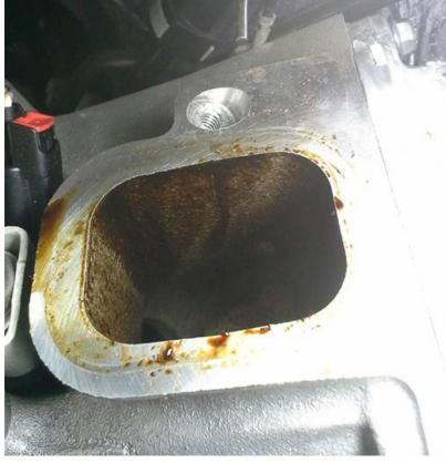
If this is found the cylinder head will need to be replaced.
