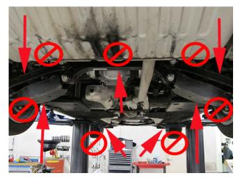
When recovering or transporting a Cadillac ATS, the under vehicle components may be damaged if the recommended towing and securing steps are not followed.
