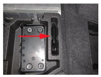
3.1. Locate the recovery tow eye, secured in the rear compartment storage area.
