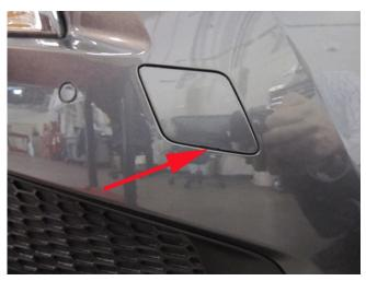
3.2. Carefully open the cover in the front or rear fascia by using the small notch that conceals the tow eye socket. Use care to not damage the paint.
