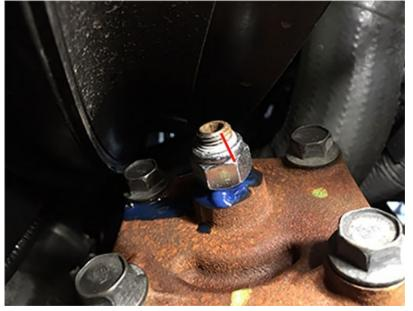
6. Using an Allen wrench, tighten the adjuster stud (turning clockwise) until the nut bottoms out on the cover plate, shown below.
