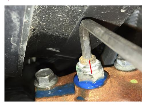
7. Using a torque wrench with crow foot & Allen wrench, turn the adjuster stud and nut simultaneously while torquing to 68 lb ft (92 Nm). Make sure the mark or scribe on the adjuster stud and nut (made during step 2) are still in alignment. If not, slightly loosen the nut, realign the marks, and retorque.
