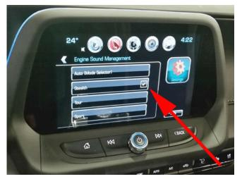
4. Lower the vehicle. Press and release the ignition mode switch to put the vehicle in the Accessory mode. The amber LED will illuminate once the correct mode has been achieved. From the home page of the radio, follow the path listed below to turn the vehicle's Stealth mode on. Settings>Driving Mode>Engine Sound Management>Stealth. This will close the valves to simplify applying epoxy to one side of valve.
