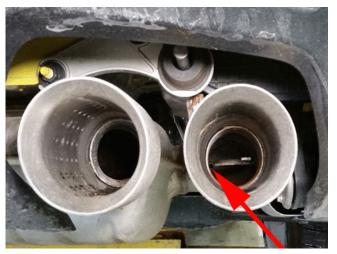
**3.** Using brake parts cleaner and a long wire brush, clean the ceramic pins on each side of each valve.
