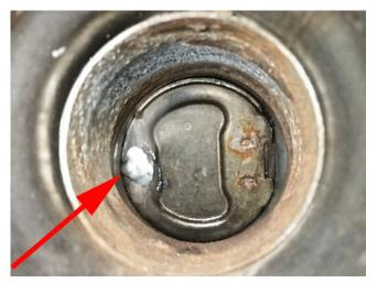
5. Raise the vehicle back in the air and using a long Q-Tip taped to a long handled screwdriver, apply epoxy to the ceramic pin where it meets the exhaust valve.
