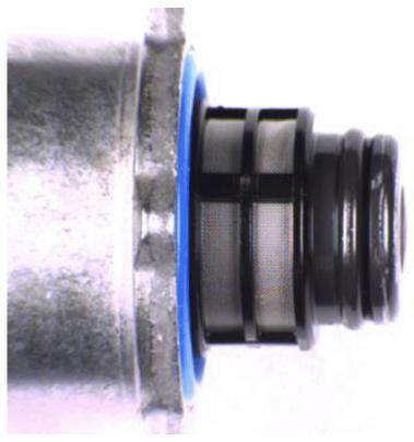
If Pressure Regulator 1 has no debris that can be picked up with a magnet on the screen, continue with Fuel Injection Pump replacement.
