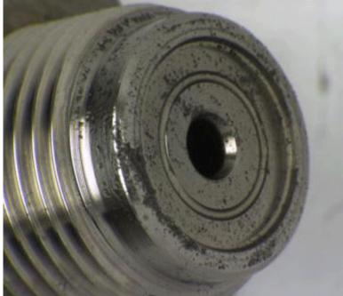
If additional debris that can NOT be picked up with a magnet (Contamination) is found on the Fuel Pressure Regulator 1, Fuel Rail Pressure Sensor, and/or Fuel Pressure Regulator 2 (Pressure Relief Valve), refer to PIP5370 and Contaminants-in-Fuel Diagnosis. DO NOT perform the repair listed in this bulletin.
