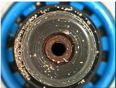
If there are only a few pieces of debris that can be picked up with a magnet found on Pressure Regulator 1, remove the Fuel Rail Pressure Sensor and/or Fuel Pressure Regulator 2 (Pressure Relief Valve) for inspection.
