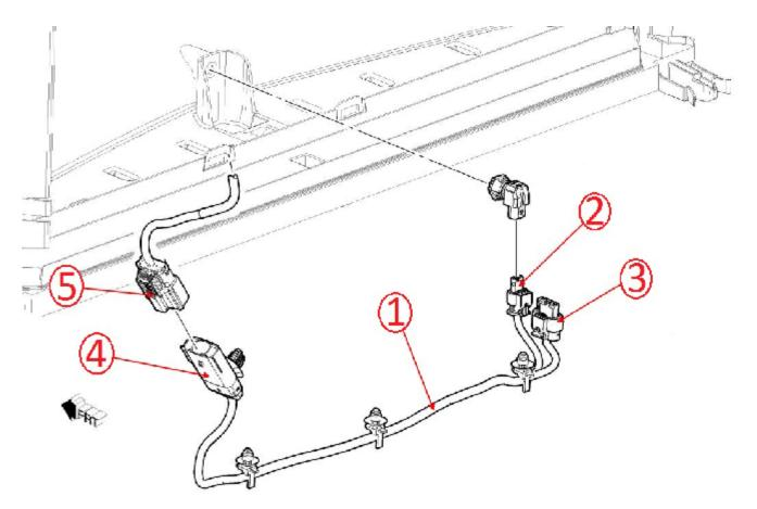
Inspect the Ambient Air Temperature Sensor Wiring Harness connectors B9 (2), M60B (3) and the X119 (4, 5) for any signs of corrosion.
