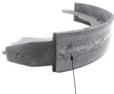
Acceptable Hairline Cracks
