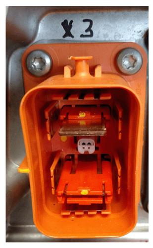
Connectors need to be square to each other before the cam lock is engaged.
