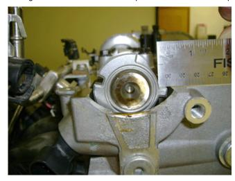
**Notice:** Each of the procedures above may not detect a small movement in the reluctor, it may be necessary to compare to a known good engine if in doubt. Also note that the cam cover gasket surface does not line up with the same face/slot on the intake and exhaust reluctor.
