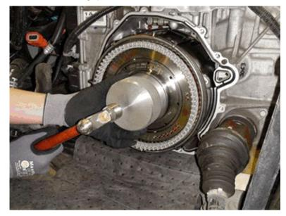
Please also order and replace the rotor shaft seal this could be damage during bearing removal or installation
