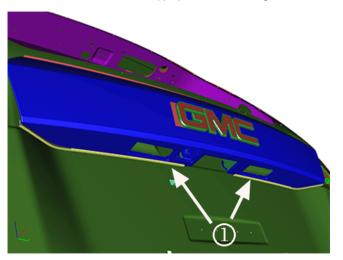
When repairing this rust spot condition, a new two-piece insulator service part (1) should be installed between the applique and the liftgate.
