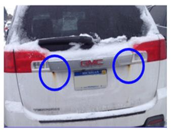
On some vehicles, due to the applique contacting and rubbing on the liftgate painted surface, rust spots (shown circled above) may be evident at the lower corners of the center chrome applique on the rear liftgate.
