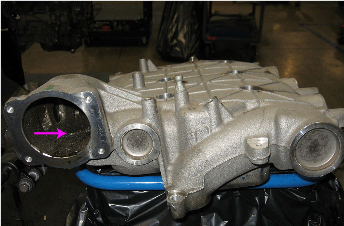
View of Debris in Aluminum Intake Manifold — Ports to Cylinder Heads
